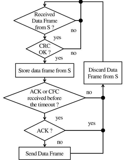
Fig. 8. Flow chart at a potential relay T.
